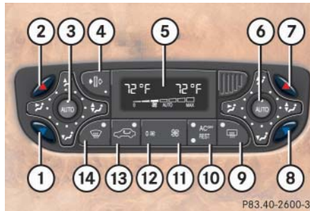
Automatic climate control panel
